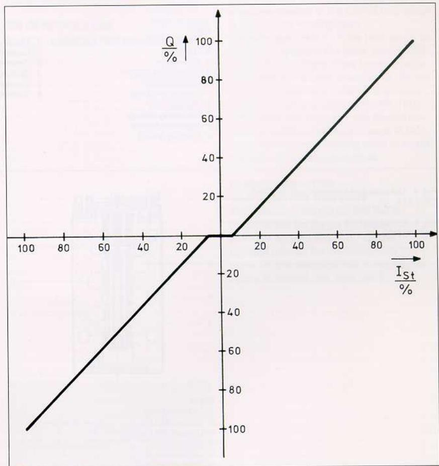
Fig. 7. Flow curve of TR-h 7 / S related on pressure drop of 10 bars.  $Q$  = flow rate (standard rates see page 8, table 2.  $I_{st}$  = control current ( $100\% \hat{=} 300$  mA across one coil).
