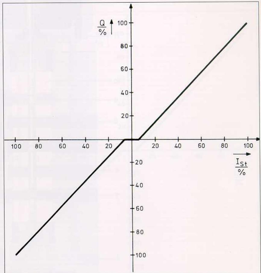
Fig 10. Flow curve of TR-h 7 / .F related on pressure drop of 10 bars. Flow rate for pressure drop  $P_x$  is to be calculated by  $Q_x = Q \sqrt{\frac{\Delta P_x}{10}}$
