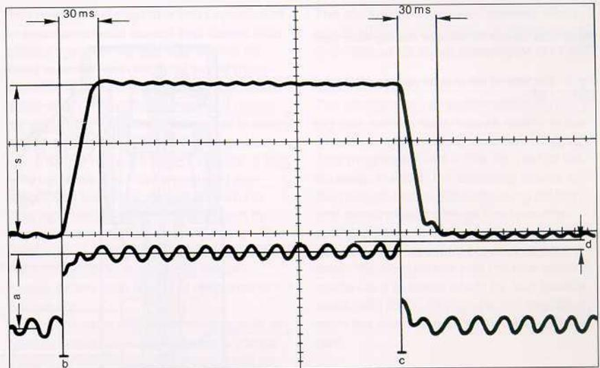
Fig. 6 Transient response characteristic stroke  $s =$  vs time  $t$  of TR-h 7 / S and TR-h 7 / SE at 20 bars; a = control current, b = on, c = off, d = dither 25 mA
