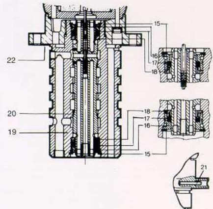
Assembly is carried out in the reverse order. All throttles and channels should first be thoroughly cleaned. The sliding surfaces of the pilot piston and the control piston must be glossy and free from grooves. For assembly cleanliness is extremely important.
