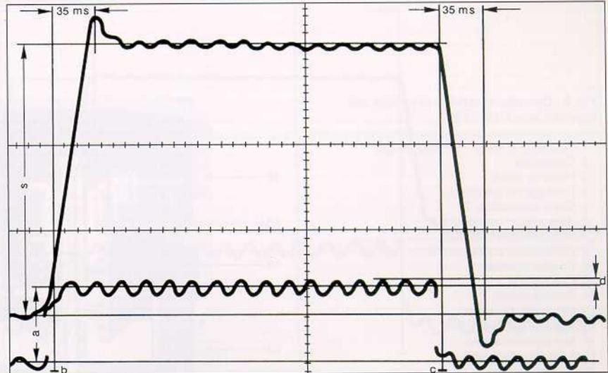
Fig. 9 Transient response characteristic stroke  $s = vs$  time  $t$  of TR-h 7 / F at 35 bars; a = control current, b = on, c = off, d = dither 25 mA
