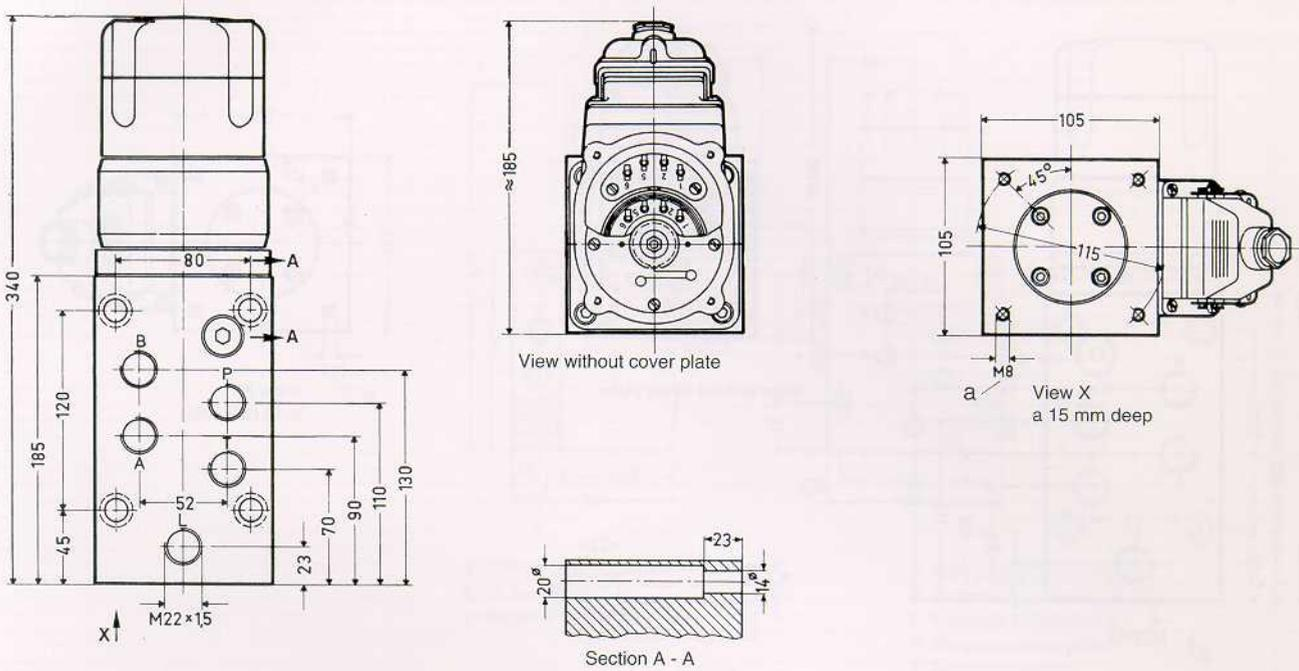
Fig. 14 Dimensions of TR-h 7 / SE
